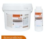
**Technical data:** Mixing ratio: 8:1 by weight. Processing/laying time: 50-60 min. Fit for walking on after: 4-6 h. Fit for further work after: 12 h. Final hardness after: 48 h. Flash-off time: no. Suitable for in-floor heating: yes. All data are based on standard climate (23°C and 50% rel. humidity). If the conditions differ from this standard, the times will differ too!
